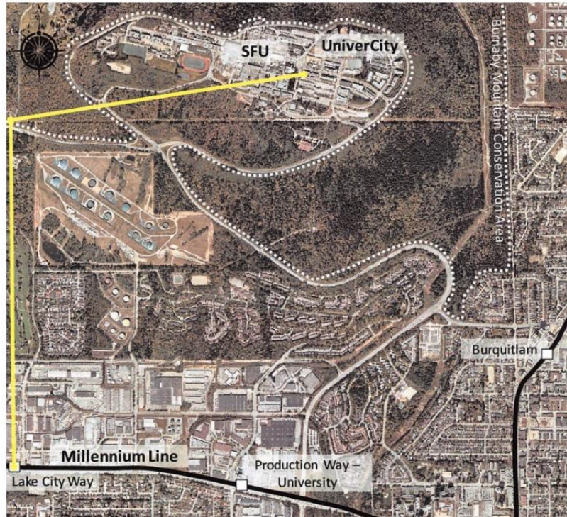
Figure 3: Gondola route from Lake City Way SkyTrain station to SFU with midway station
